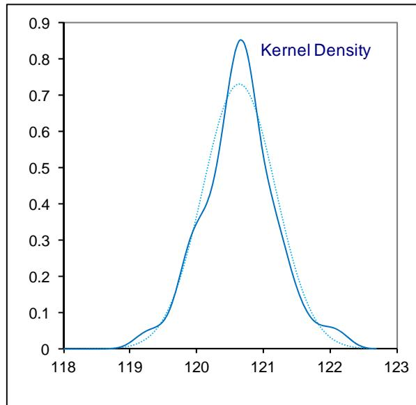
Determination of Kinematic Viscosity @ 100°C on sample #14083; results in mm<sup>2</sup>/s
