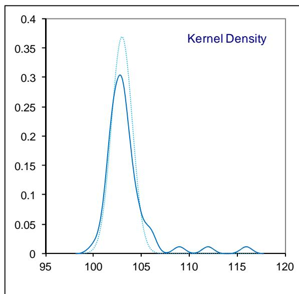
Determination of Kinematic Viscosity @ 40°C (Houillon) on sample #14083; results in mm<sup>2</sup>/s
