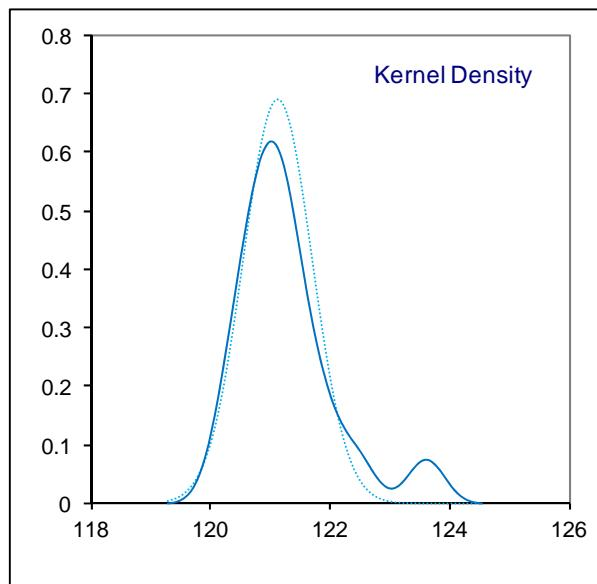
Determination of Kinematic Viscosity @ 100°C (Houillon) on sample #14083; results in mm<sup>2</sup>/s
